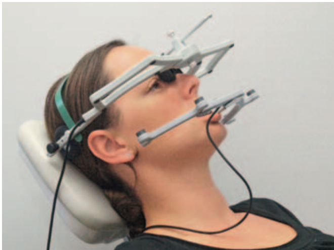
Fig 2 Example of an ultrasound-based electronic movement recording system (JMA – Jaw Motion Analyzer, Zebris) (Photo ©dentaConcept Verlag).
