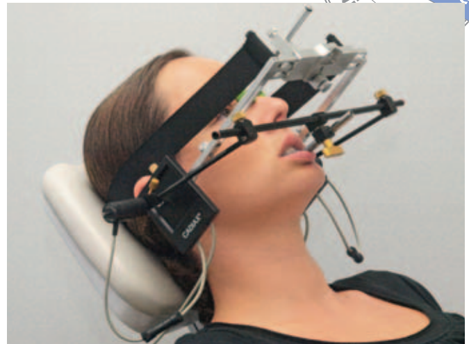
Fig 3 Example of an electronic movement recording system based on the voltage division method (Cadiax Compact 2, Gamma Dental) (Photo ©dentaConcept Verlag).
